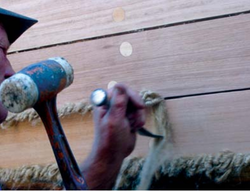
Caulking new planks in Derwent Hunter's hull during her 2006 refit
